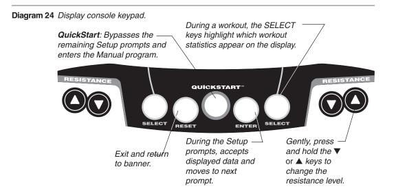
The following information explains the different uses of the keys from left to right. To locate each key, look at the display console or refer to Diagram 24.
